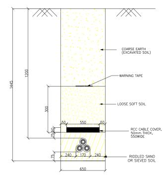
Figure 1.9 – 66kV Buried Cable for Single Circuit
