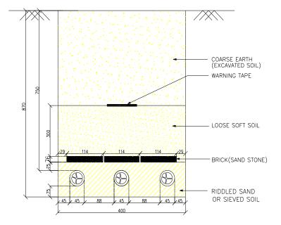
Figure 1.1 – 1.1kV, 150sqmm Buried Cable
