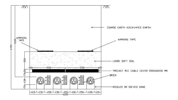
Figure 1.11 – 66kV 3Cx300 sq mm Four No's Cable Runs
