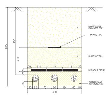
Figure 1.2 – 1.1kV, 300sqmm Buried Cable
