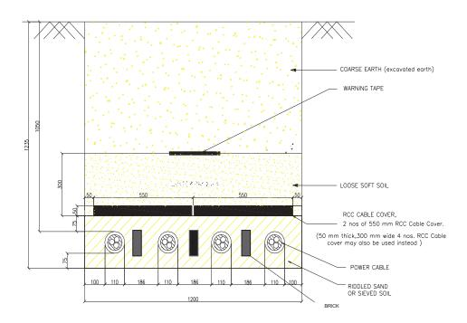
Figure 1.8 – 33kV Buried Cable Option-2 for Four Circuits
