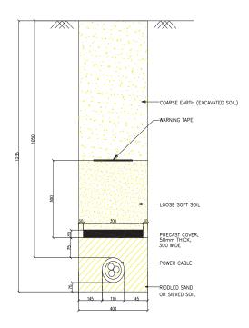
Figure 1.5 – 33kV Buried Cable for Single Circuit
