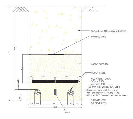
Figure 1.6 – 33kV Buried Cable for Double Circuit
