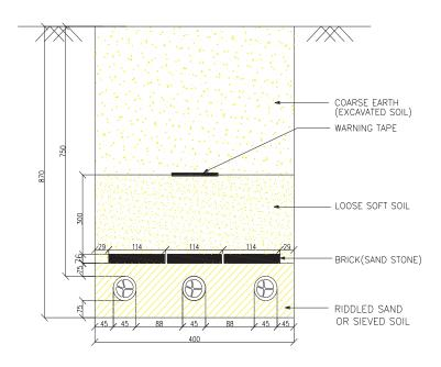
Figure 1.1 – 1.1kV, 150sqmm Buried Cable
