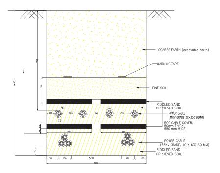
Figure 1.10 – 66kV Double Circuit and 11kV Circuits
