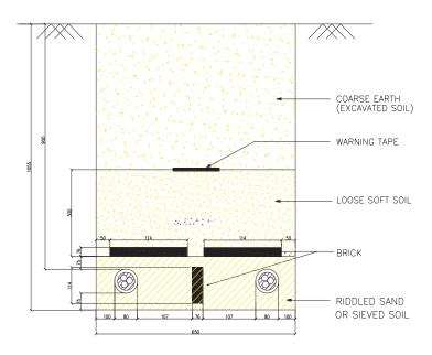
Figure 1.4 – 11kV Buried Cable for Double Circuit
