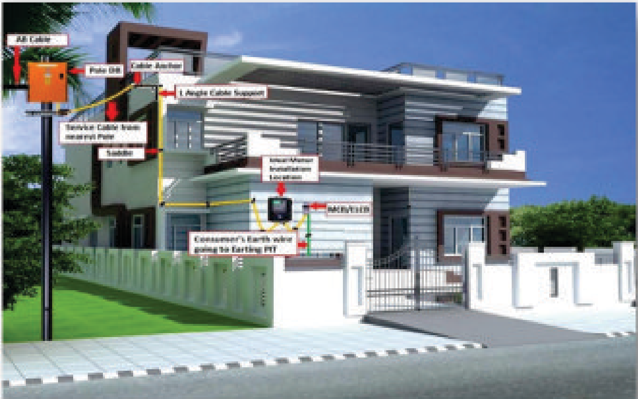
Photograph 1: An overview of Electrical connectivity between Pole and Meter at Consumer House
