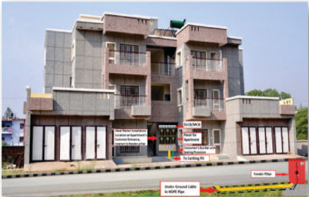
Photograph 2: An overview of Electrical connectivity between Feeder pillar and Consumer panel in Apartments
