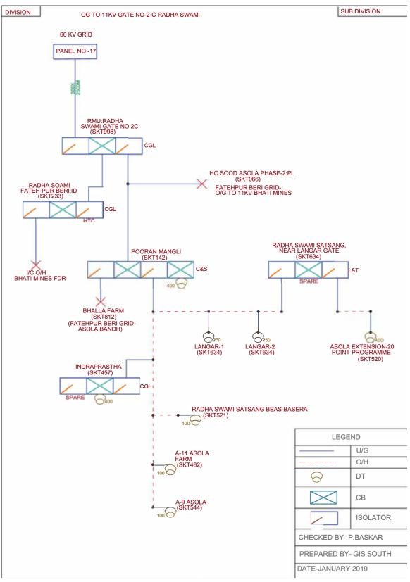
Figure 4: SLD of 11 kV Radha Soami feeder
