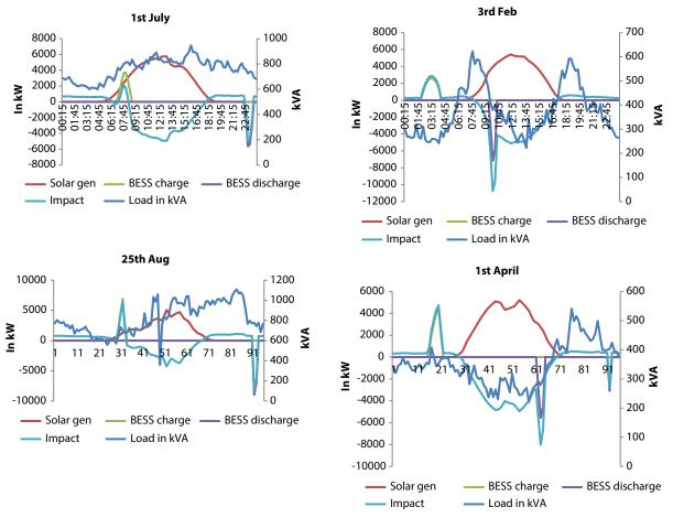
Figure18: Impact on feeder-level loading as a result of operations of microgrids
