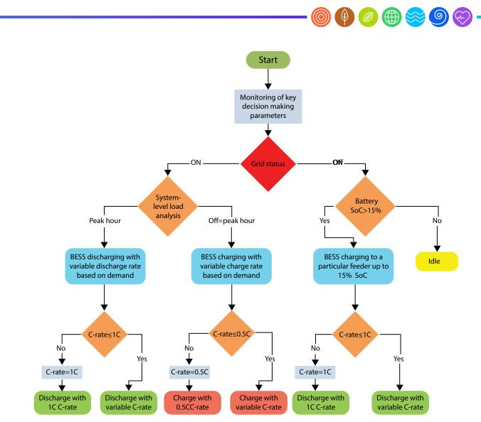
Figure 14: Basic control methodology for BESS operation
