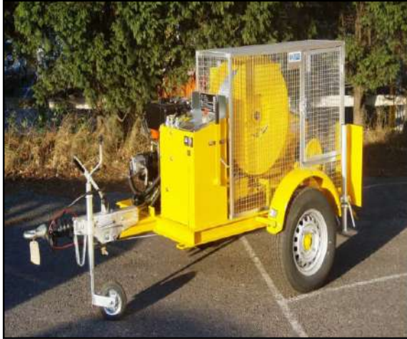
(Cable roller pulling machine)
