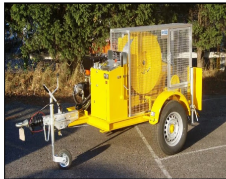
(Cable roller pulling machine)
