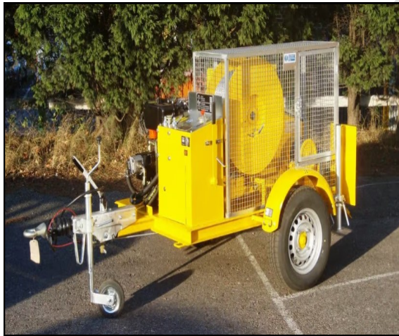
(Cable roller pulling machine)
