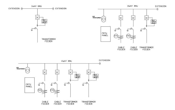
a) 11kV RMU shall have Feeder Circuit breaker (FCB) and Transformer circuit breakers (TCB) all are motorized
