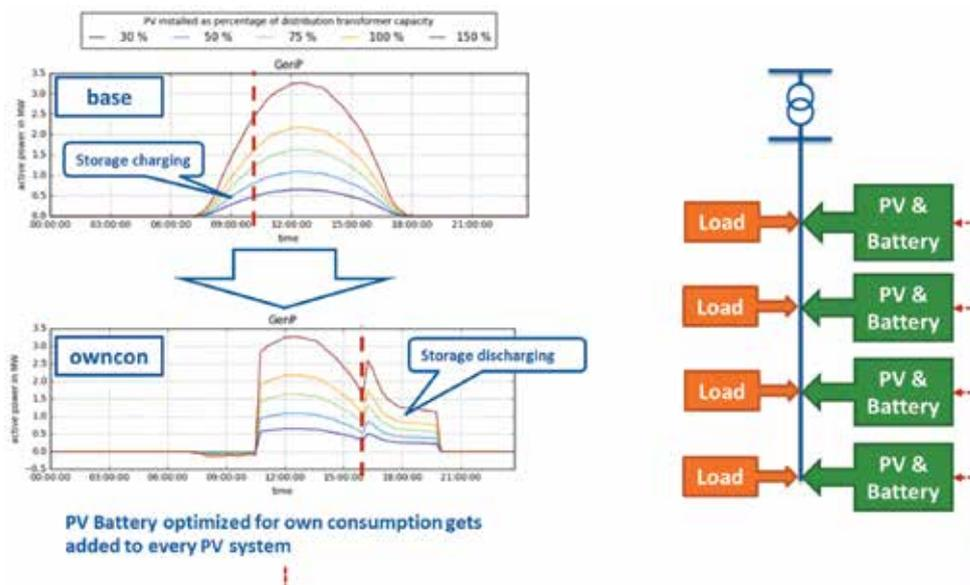
**Figure 3: PV Battery implementation with own consumption optimization**
