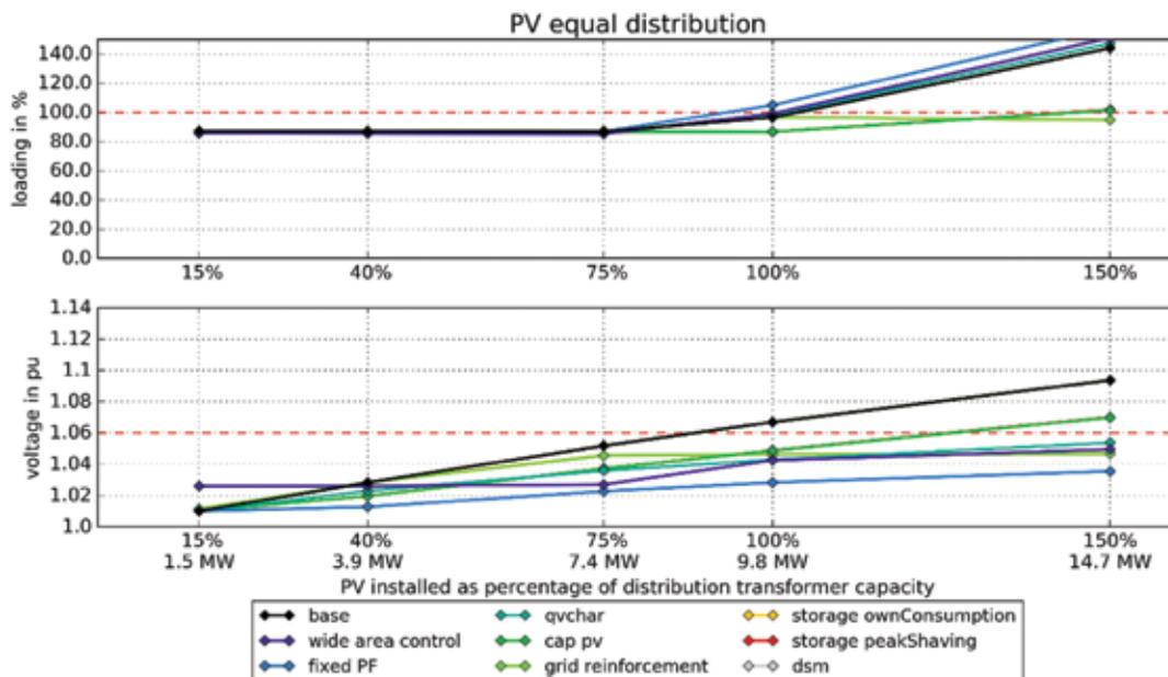
**Figure 6: Simulation results of the rural feeder with two parallel MV feeders and equal PV distribution.**
