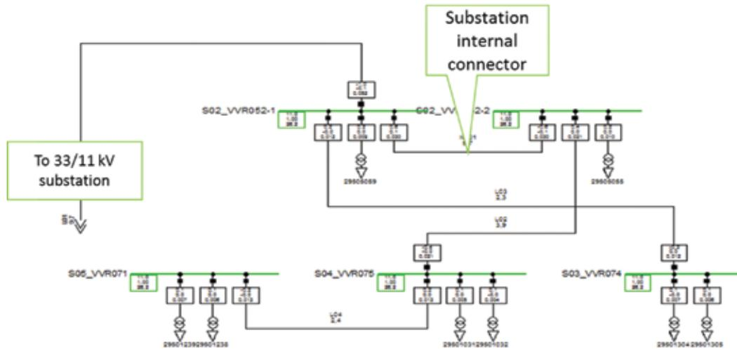
**Figure 1: PowerFactory Single-Line-Diagram of 11 kV feeder.**
