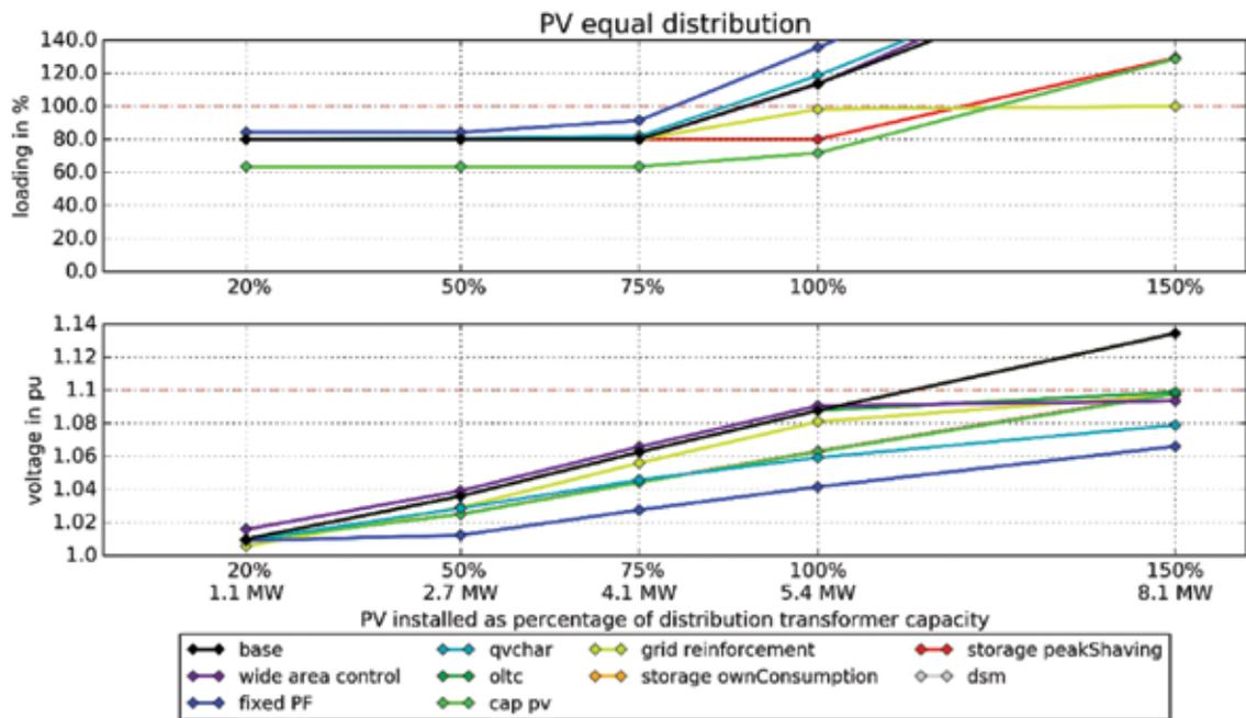
**Figure 5: Simulation results for urban feeder with LV network and equal PV distribution.**
