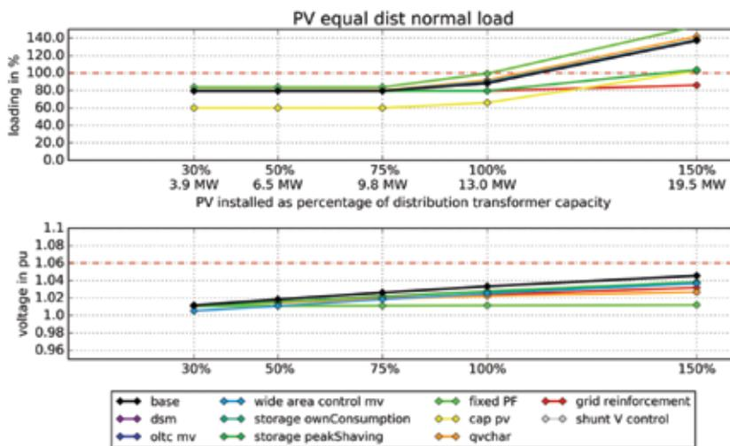
**Figure 7: Simulation results for the urban feeder in Bhopal with rooftop photovoltaic plants equally distributed along the feeder with normal load considered**
