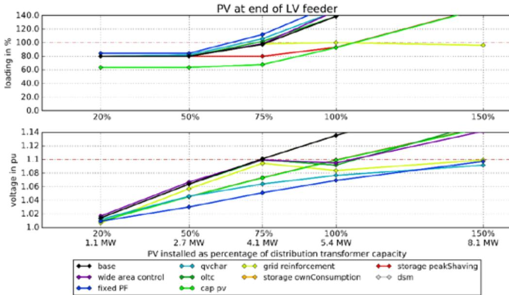
**Figure 61: Simulation results for urban feeder with LV network and PV at the end of the feeder.**
