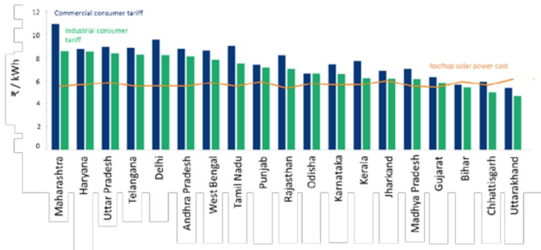
Figure 18: Grid parity of rooftop PV in selected Indian states, 2016. [50]
