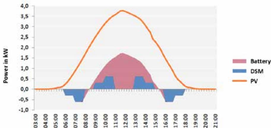
**Figure 8: Optimized operation of PV, battery and household demand side management, as developed by Energynautics for the distribution grid study in the German federal state of Rhineland-Palatinate. [38]**
