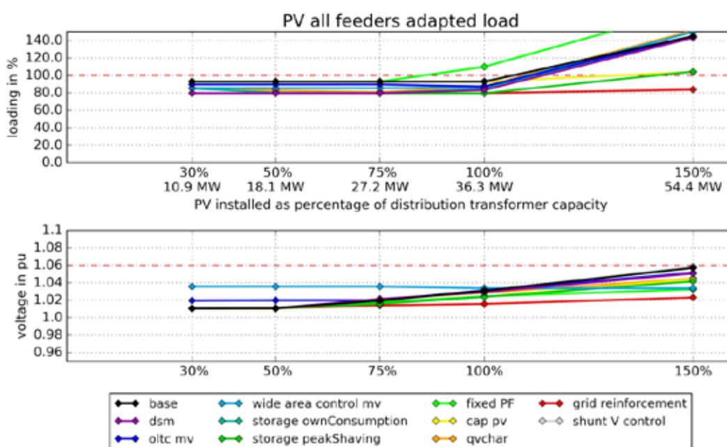
**Figure 76: Simulation results for the rural feeder in Bhopal with rooftop photovoltaic plants equally distributed along the feeder with adapted load considered**
