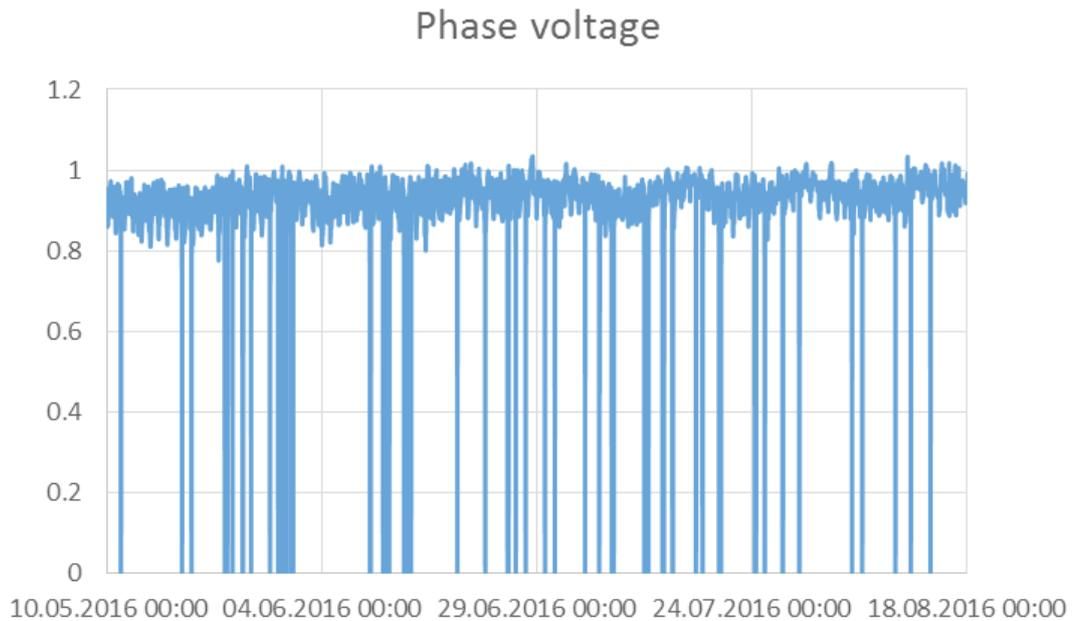
**Figure 35: Voltage measurements of the secondary (400 V) of a distribution transformer in rural Delhi, showing gaps as well as voltage frequently dropping below 0.9 p.u.**
