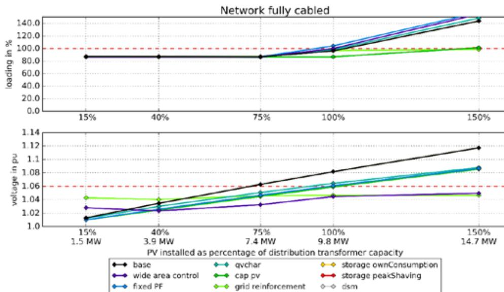
**Figure 69: Simulation results of the rural feeder with two parallel MV feeders and equal PV distribution with the network fully cables.**
