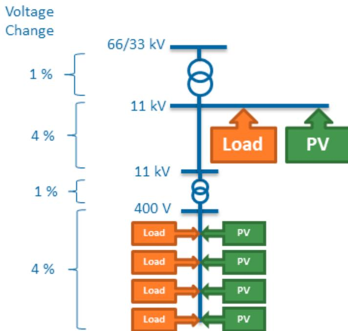
Figure 41: Voltage profile / tolerances Delhi.
