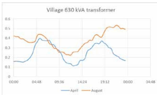
**Figure 29: Load data for a transformer supplying a part of a village on a rural feeder for a day in April and one in August.**
