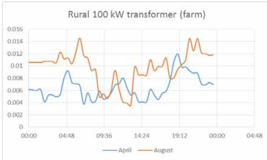
**Figure 30: Load data for a transformer supplying a farm on a rural feeder for a day in April and one in August.**
