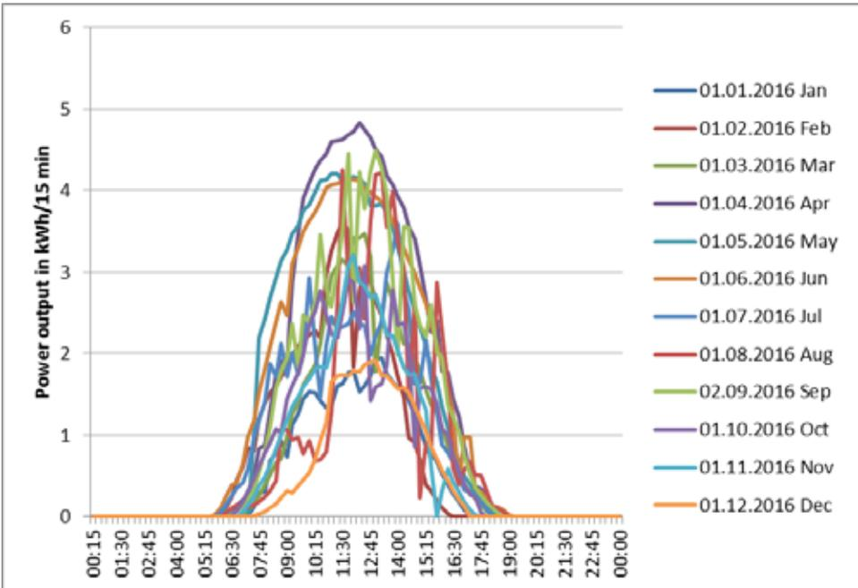
Figure 39: Output of a 25 kWp PV installation in Delhi for the first day of each month. Nominal output would be 6.25 kWh/15 min.
