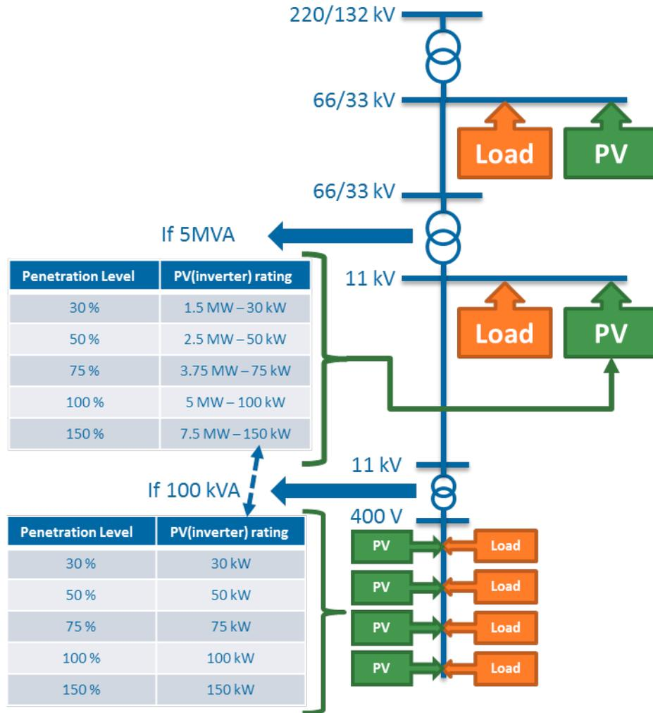
**Figure 43: Consideration of Impact of Parallel feeders**
