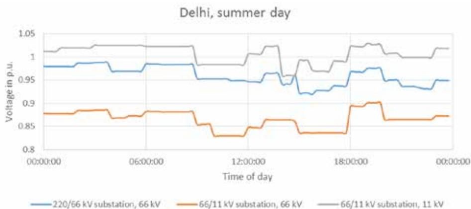
**Figure 34: Voltage measurements of 66 and 11 kV level grids in urban Delhi, summer day. Tap positions (66/11 kV) are switched during the day.**
