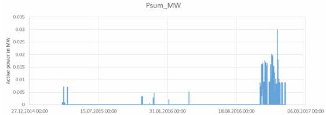
**Figure 24: Distribution transformer data from a rural feeder, rendered unusable by very large gaps.**
