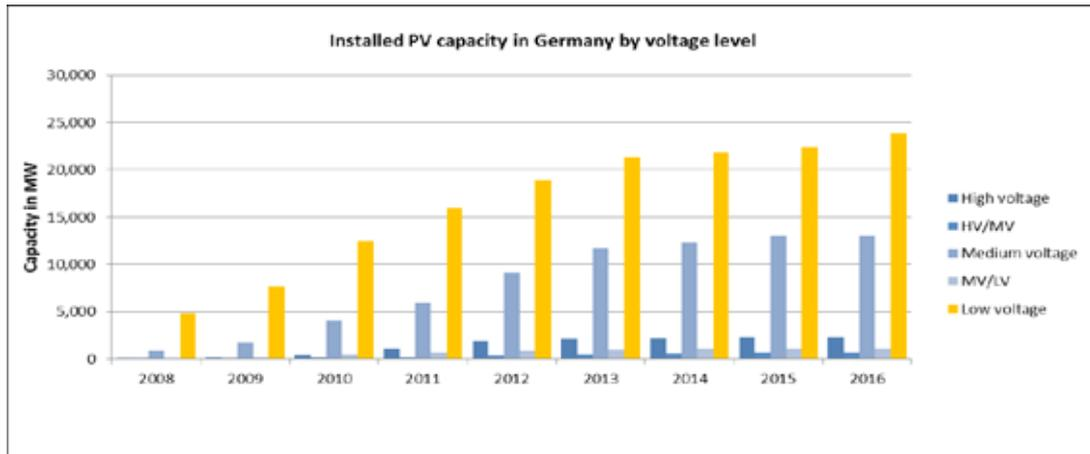
Figure 3: Development of installed PV capacity in Germany by voltage level of connection. [23][24]
