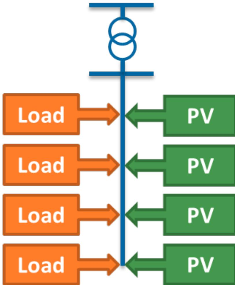
Figure 44: Rooftop photovoltaic plants equally distributed along feeder
