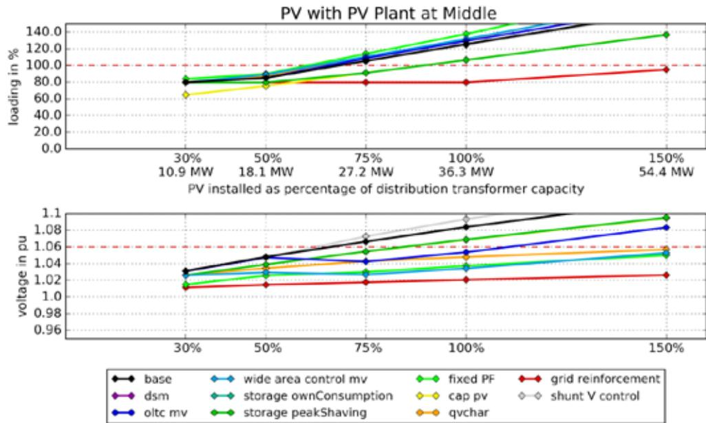
Figure 78: Impact of reactive power injection through the utility scale solar plant at the middle of the feeder
