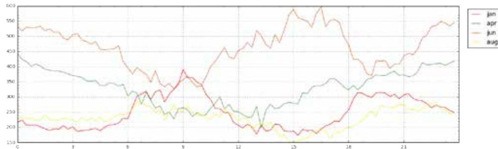
**Figure 28: Daily load profiles of an urban 11 kV feeder in Bhopal from the first day of each month.**
