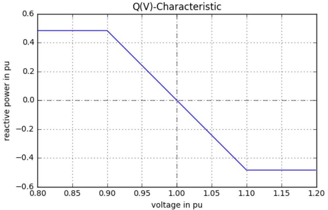
**Figure 52: Utilized Q-V-characteristic.**
