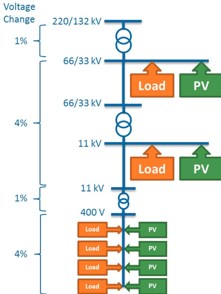
Figure 40: Voltage profile / tolerances Bhopal.
