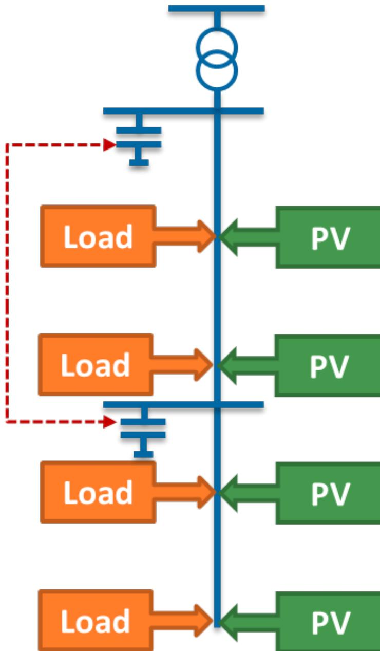
**Figure 51: Shunt Compensator for voltage control**
