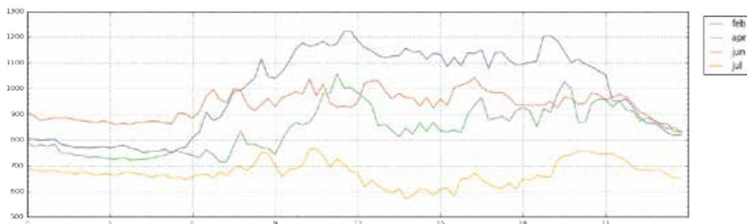
**Figure 32: Daily load profiles of a rural 11 kV feeder in Bhopal from the first day of each month.**
