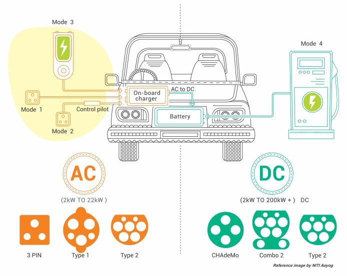
AC and DC charging are further classified into four charging modes, with Modes 1-3 pertaining to AC charging and Mode 4 pertaining to DC charging. Modes 1 and 2 are applicable for connecting an EV to a standard socket outlet, utilizing a cable and a plug.
